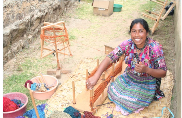
Maria warps a scarf on a warping board. The warp is the vertical threads.
